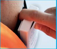
**PRESSTOCHECK<sup>™</sup>** - Press the front and backs of both filter covers together to stop air from entering through the filters.
